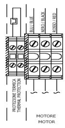
The motor cable must be a shielded cable with 3 poles + earth + shielding.
