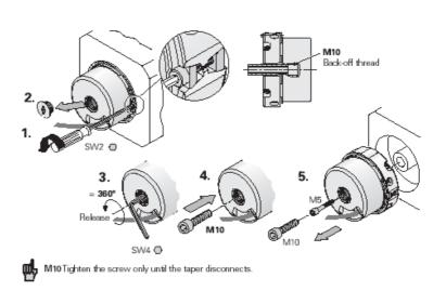
Before installing the replacement encoder make sure it is entirely interchangeable with the previous one.
