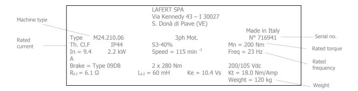
$R_{f-f}$  = resistance on winding terminals (phase-to-phase)  $[\Omega]$
