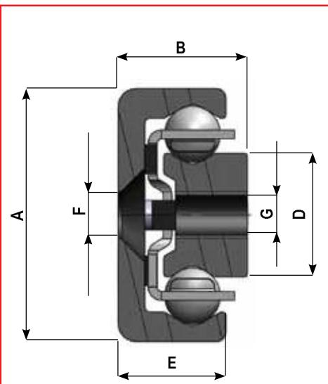
The semi-telescopic slides SR28 allow for a stroke H, equal to half the length of the slide, plus a minor stroke 10-25mm depending on type.
