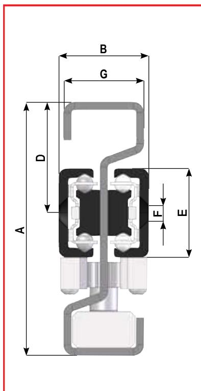
The TSH..DSY with synchronized movement for both single and double stroke, is composed of two semi-telescopic slides SR that move together, as connected by an integrated rack & pinion system. Hereby moving the intermediate element 500mm the mobile part extends 1000mm.
